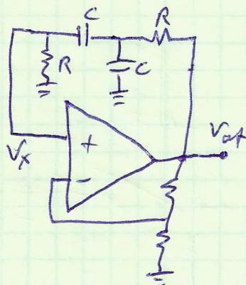
$$\frac{V_{out}}{V_x} = \frac{(1+SCR) + (2+SCR)(SCR)}{SCR}$$
