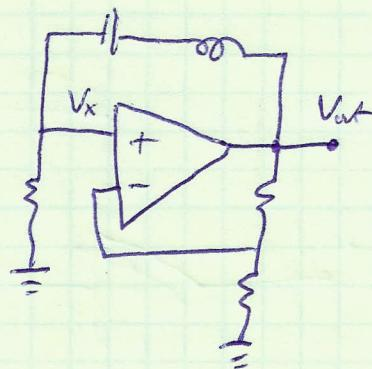
$$B = \frac{-V_x}{V_{out}} = \frac{-R}{R + sL + \frac{1}{sC}}$$
