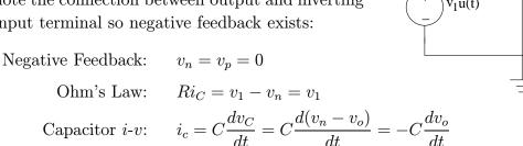
Substituting for  $i_C$  from Ohm's law into capacitor *i*-*v* equation, and integrating the resulting equation we get:
