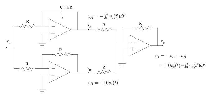
**Example:** Design an OpAmp circuit which solves the differential equation:  $\frac{d^2v_o}{dt^2} + 2\frac{dv_o}{dt} + v_o = v_s(t).$
