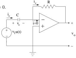
Negative Feedback:  $v_n = v_p = 0$ Ohm's Law:  $Ri_C = v_n - v_o = -v_o$ Capacitor *i*-*v*:  $i_c = C \frac{dv_C}{dt} = C \frac{d(v_1 - v_n)}{dt} = C \frac{dv_1}{dt}$
