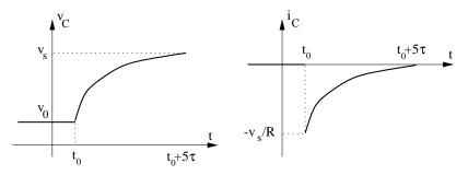
If the switch was closed at time  $t = t_0$  instead of time zero, the capacitor voltage waveform would be (let  $t' = t - t_0$  and switch closing at t' = 0):
