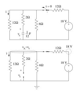
No-jump condition leads to the initial condition for t > 0:  $v_C(0^+) = v_C(0^-) = 4.5$  V. Note that although we like to find *i*, the initial condition is obtained for  $v_C$  as no-jump condition only applies to  $v_C$  and *i* may have a discontinuity at the switching time.
