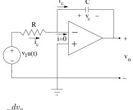
**Example 4: Differentiator:** Find  $v_o$  if  $v_C(t = 0) = 0$ . We replace the OpAmp with its circuit model. As the current flowing into the OpAmp is zero, the current in the resistor is the same as  $i_C$ . We also note the connection between output and inverting input terminal so negative feedback exists:
