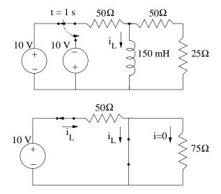
No-jump condition leads to the initial condition for t > 1:  $i_L(t = 1^+) = i_L(t = 1^-) = 0.2$  A. We now proceed to solve t > 0 circuit:
