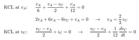
where we substituted for  $i_C$  from the capacitor *i*-*v* equation. The above are two equations in our two node-voltages  $v_A$  and  $v_C$ . Substituting for  $v_A$  from first into the second, we get:
