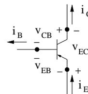
The above model is called a “large signal” model as it applies to any size currents/voltages applied to the BJT (as opposed to a “small-signal” model discussed later). In addition, this is a “low-frequency” model as the junction capacitances are NOT taken into account (you will see high-frequency transistor models in ECE102). PSpice uses the Ebers-Moll model which includes a better treatment of transistor operation in the saturation mode.
