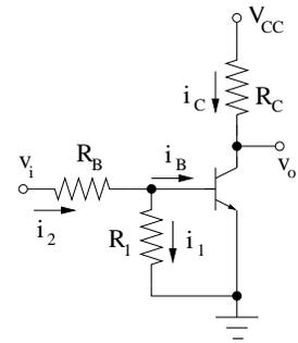
$$i_1 = \frac{v_{BE}}{R_1} \quad i_2 = i_B + i_1 \approx i_1 = \frac{v_{BE}}{R_1}$$
