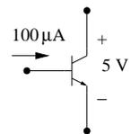
**Problem 4.** In circuit below find  $v_{EB}$ ,  $i_C$ ,  $v_{EC}$ , and state of the transistor (Si BJTs with  $\beta = 100$ ).
