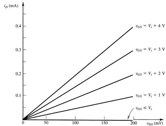
The slope of  $i_D$  versus  $v_{DS}$  line is the conductance of the channel. For  $v_{GS} \leq V_t$  no channel exists (zero conductance). As value of  $v_{GS} - V_t$  increases, channel becomes wider and its conductivity increases (because its  $n$ -type charge concentration increases). Therefore, the channel conductance (slope of  $i_D$  versus  $v_{DS}$  line) increases with any increase in  $v_{GS} - V_t$  as is shown above.
