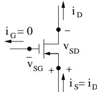
**Cut-off:**  $v_{SG} < |V_{tp}|, \quad i_D = 0$
