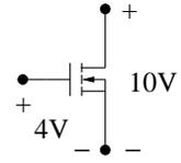
**Problem 17.** In circuit below find  $v_{SG}$ ,  $i_D$ ,  $v_{SD}$ , and state of the transistor (Use  $k'_n(W/L)_n = k'_p(W/L)_p = 0.4 \text{ mA/V}^2$ ,  $\lambda = 0$ ,  $V_{tn} = 3 \text{ V}$  and  $V_{tp} = -3 \text{ V}$ ).
