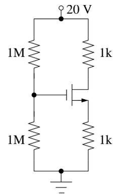
Negative root is unphysical so  $v_{GS} = 6.92$  V. GS-KVL give  $i_D = 3.08$  mA. DS-KVL gives  $v_{DS} = 20 - 6.16 = 13.8$  V Since  $v_{DS} = 13.8 > v_{GS} - V_{tn} = 6.92 - 3 = 3.92$  V, our assumption of NMOS in saturation is justified.
