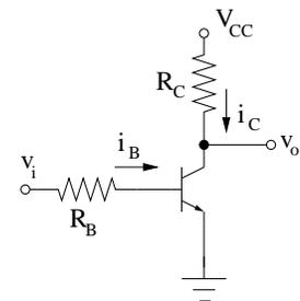
To find the transfer function of this gate, we need to find  $v_o$  for a range of  $v_i$  values. This plot will also help identify the values of  $v_{IL}$  and  $v_{IH}$ .
