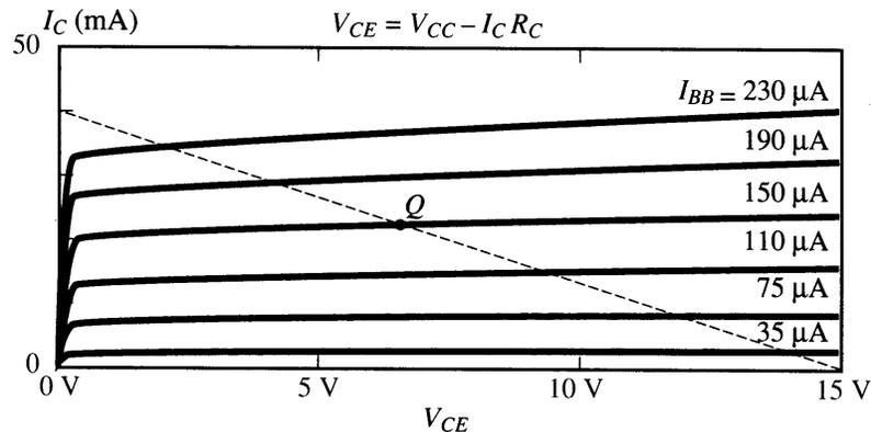
Note that if an emitter resistor is present (*e.g.*, Example 3 in page 3-8), the load line can still be constructed noting that  $i_E = [(\beta + 1)/\beta]i_C \approx i_C$ :
