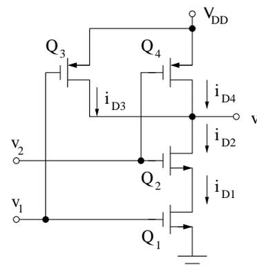
above, we have  $v_o = v_{DS1} + v_{DS2} = V_{DD}$ . This gives  $v_{DS1} = V_{DD}$  and  $v_{GS2} = v_2 - v_{DS1} = 0 - V_{DD} = -V_{DD} < \bar{V}_t$ , a contradiction of Q2 being ON. Therefore, Q2 should be OFF.
