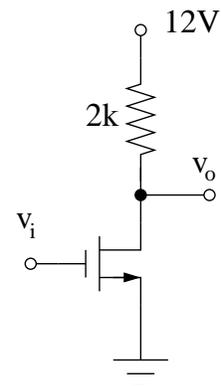
B)  $v_i = 12$  V. From GS-KVL, we get  $v_{GS} = 12$  V. Since  $v_{GS} > V_{tn}$ , NMOS is not in cut-off. Assume NMOS in saturation mode. Then:
