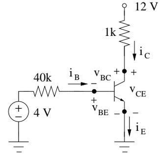
**Example 2:** Compute the parameters of this circuit ( $\beta = 100$ ).
