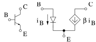
We can also construct a circuit model for a BJT which is valid for cut-off and active modes.
