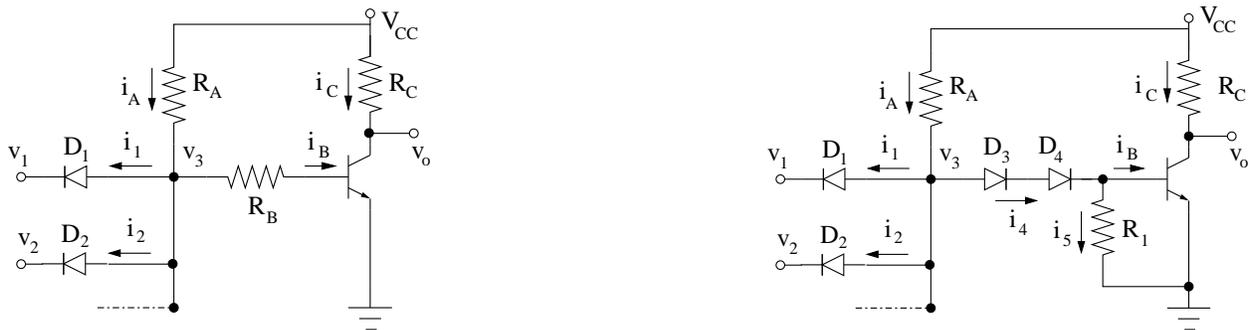
**Example:** Verify that the DTL circuit above (with  $R_A = 5 \text{ k}\Omega$ ,  $R_C = 1 \text{ k}\Omega$ ,  $R_1 = 5 \text{ k}\Omega$ , and  $V_{CC} = 5 \text{ V}$ ) is a NAND gate. Assume that “low” state is 0.2 V, “high” state is 5 V, and BJT  $\beta_{min} = 40$ .
