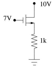
**Problem 21.** In circuit below find  $v_{GS}$ ,  $i_D$ ,  $v_{DS}$ , and state of the transistor (Use  $k'_n(W/L)_n = k'_p(W/L)_p = 0.4 \text{ mA/V}^2$ ,  $\lambda = 0$ ,  $V_{tn} = 3 \text{ V}$  and  $V_{tp} = -3 \text{ V}$ ).
