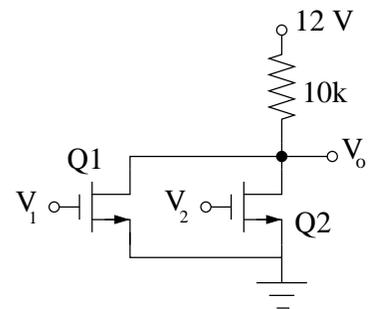
Case 1:  $v_1 = v_2 = 0.2$ . Since  $v_{GS1} = 0.2 < V_{tn} = 1$  and  $v_{GS2} = 0.2 < V_{tn} = 1$ , both transistors will be in cut-off:  $i_{D1} = i_{D2} = 0$ . Then,  $i_1 = i_{D1} + i_{D2} = 0$  and from KVL,
