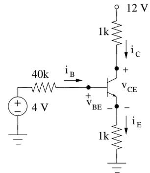
So BJT is not in cut off and  $v_{BE} = 0.7 \text{ V}$  and  $i_B > 0$ . Here, we cannot find  $i_B$  right away from BE-KVL as it also contains  $i_E$ . Assume BJT is in active linear,  $i_E = (\beta + 1)i_B$ :
