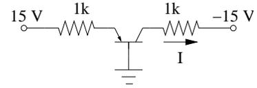
Assume BJT (NPN) is OFF,  $i_B = i_C = i_E = 0$  and  $-v_{BE} < 0.7$  V. BE-KVL gives:
