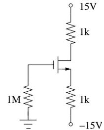
Assume NMOS is in cut-off:  $i_D = 0$ ,  $v_{GS} < V_{tn} = 3$  V.
