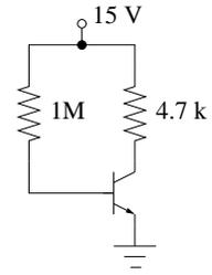
**Problem 6.** In circuit below find  $v_{EB}$ ,  $i_C$ ,  $v_{EC}$ , and state of the transistor (Si BJTs with  $\beta = 100$ ).
