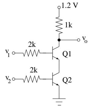
Case 1:  $v_1 = 0.4, v_2 = 0.4$ : Assume Q2 is off ( $i_{B2} = 0, v_{BE2} < V_{D0}$ ). Substituting for  $i_{B2} = 0$  in the BE2-KVL above, we get:  $v_{BE2} = v_2 = 0.4 < 0.7 = V_{D0}$ . Thus, Q2 is off and  $i_{C2} = 0$ . Since  $i_{E1} = i_{C2} = 0$  and  $i_{E1} = i_{C1} + i_{B1} = 0$ , we should have  $i_{C1} = 0$  (because  $i_{C1} \geq 0$  and  $i_{B1} \geq 0$ ). Then, from CE-KVL above:
