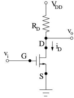
This is a quadratic equation in  $v_{DS}$ . The two roots are:  $v_{DS} = 2.2$  V and  $v_{DS} = 21.8$  V. The second root is not physical as the circuit is powered by a 12 V supply. Therefore,  $v_{DS} = 2.2$  V. As  $v_{DS} = 2.2 < v_{GS} - V_{tn} = 10$ , NMOS is indeed in triode mode with  $v_o = v_{DS} = 2.2$  V and
