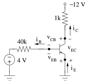
So BJT is not in cut off and BJT is ON. Set  $v_{EB} = 0.7 \text{ V}$  and use BE-KVL to find  $i_B$ .
