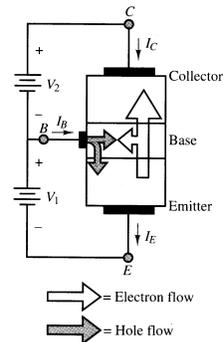
Because the BE junction acts as a diode: 1) The number of electrons that cross from the emitter into the base and diffuse into collector region depends exponentially on the voltage applied to the BE junction,  $v_{BE}$  (similar to the diode equation). 2) For a given  $v_{BE}$ , the
