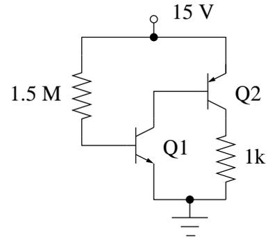
Assume Q1 is ON,  $v_{BE1} = 0.7$  V and  $i_{B1} > 0$ . BE1-KVL gives:
