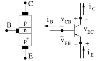
As can be seen, currents and voltages will have to reverse sign compared to a NPN transistor, *e.g.*,  $v_{EB} = V_{D0}$  for EB junction to be forward biased. As holes move slower than electrons in a semiconductor, PNP transistors have a slower response time. They are mainly used in pairs with NPN transistors, *e.g.*, push-pull amplifiers.
