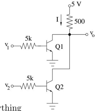
For  $v_1 = 5$  V, assume that Q1 is NOT in cut-off ( $i_{B1} > 0$  and  $v_{BE1} = V_{D0} = 0.7$  V). Substituting for  $v_{BE1} = 0.7$  in BE1-KVL, we get  $I_{B1} = 4.3/5,000 = 0.86$  mA. Since  $i_{B1} > 0$ , Q1 is indeed NOT in cut-off. Therefore,
