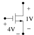
**Problem 20.** In circuit below find  $v_{GS}$ ,  $i_D$ ,  $v_{DS}$ , and state of the transistor (Use  $k'_n(W/L)_n = k'_p(W/L)_p = 0.4 \text{ mA/V}^2$ ,  $\lambda = 0$ ,  $V_{tn} = 3 \text{ V}$  and  $V_{tp} = -3 \text{ V}$ ).
