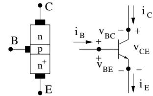
Thus, only four of these 6 parameters are independent. The relationships among these four parameters ( $i_B$ ,  $v_{BE}$ ,  $i_C$  and  $v_{CE}$ ) represent the “ $i_v$ ” characteristics of the BJT.
