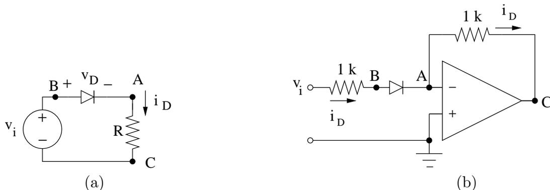
*Pspice Simulation:* Simulate circuit (a) above with  $v_i$  being a 1-kHz triangular wave with a peak to peak value of 15 V and a DC offset of  $-5\text{ V}$  (*i.e.*, input signal ranges from  $-10$  to  $+5\text{ V}$ ). Run the simulation for a few periods.
