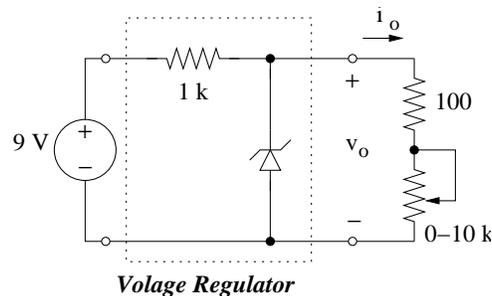
*Circuit Analysis:* Using a “Constant voltage” model for the Zener region, calculate the output voltage of the regulator ( $v_o$ ) as a function of its output current ( $i_o$ ). Estimate the maximum load current for the circuit to act as a voltage regulator.
