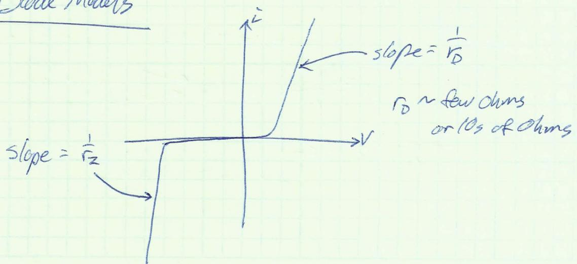
For Zener Diode, model as voltage source with resistor
