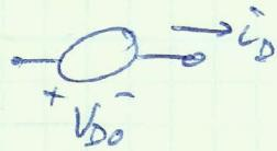
$$\text{OFF: } -V_Z < V_D < V_{D0}, i_D = 0$$
