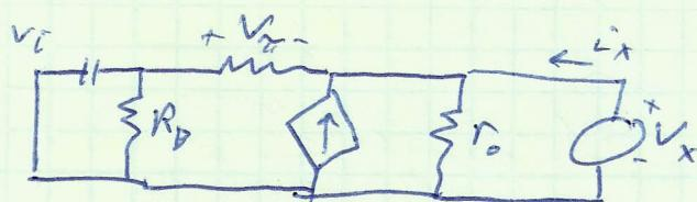
$$i_x = -g_m V_\alpha + \frac{V_x}{r_o} \times \frac{V_x}{r_\alpha}$$
