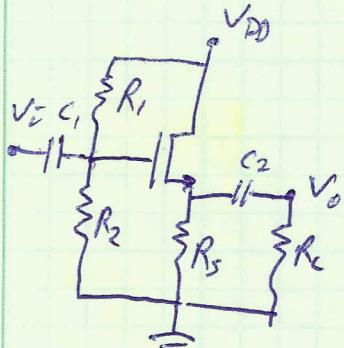
$$R_G = R_1 \parallel R_2$$
