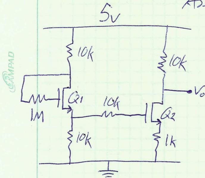
$$V_{GS2} = 1.7 \text{ V} - 1 \text{ k} \cdot I_{D2}$$
