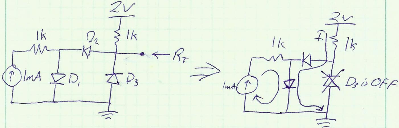
$$2V - I \cdot 1k - V_{D0} - V_{D0} = 0$$
