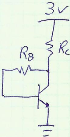
$$V_{CC} - (I_B + I_C)R_C - I_B R_B - V_{BE} = 0$$
