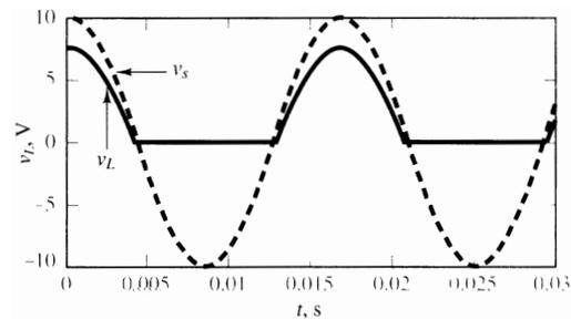
*Exercise:* Figure above right is the scope trace for a sinusoidal input waveform (dashed line) and the rectified output (solid line). Explain why the output trace does NOT EXACTLY follow  $v_o = v_i - V_{D0}$  at every point.
