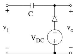
$$v_o = v_i + (V^- - V_{D0} - v_{DC})$$
