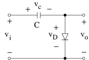
Since the two circuits are identical, we do not need to solve the clamp circuit. We use the analysis of the ideal peak detector and note that ignoring the first cycle,  $v_c = V^+ - V_{D0}$ . Thus,
