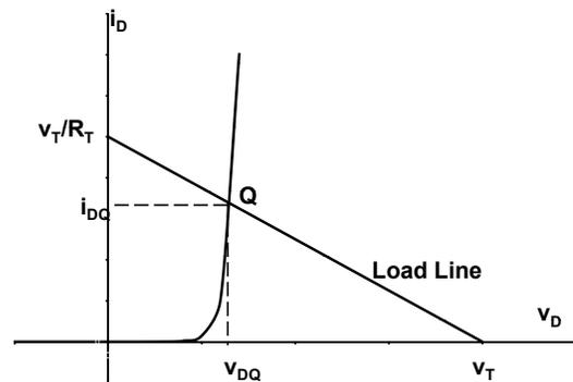
Since the solution to the above two equations in two unknowns is a pair of  $i_D$  and  $v_D$  that satisfies both equations, such a point should be both on the  $iv$  plot of the diode and on the load line, *i.e.*, at the intersection of the two. This point is called the Q-point for the Quiescent point (or the operating point) of the diode.
