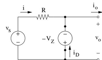
So as long as the diode is in the Zener region, the output voltage will be constant regardless of the value of  $i_o$ .
