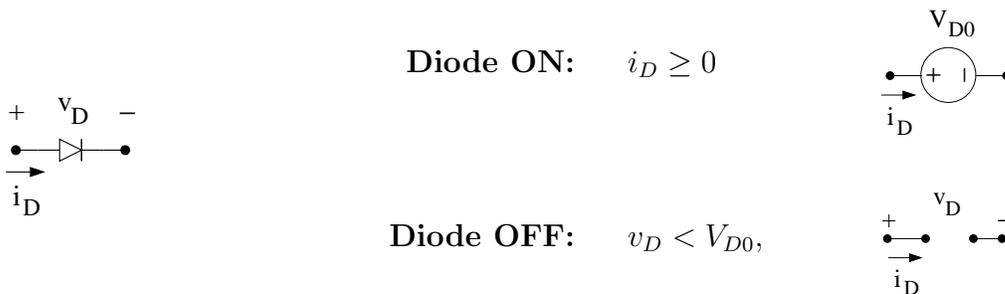
If you use the above circuit models, we need to modify our recipe for solving diode circuits accordingly:
