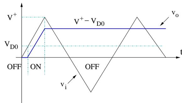
When  $v_i$  reaches its peak value,  $v_c = v_i - V_{D0} = V^+ - V_{D0}$ . After this point, the diode turns OFF because  $v_i$  is decreasing. Capacitor voltage remains at  $v_c = V^+ - V_{D0}$ .  $v_i$  eventually reaches its lowest value and start to increase again. Although  $v_i$  is increasing, the diode remains OFF because  $v_i < v_c + V_{D0} = V^+$ . Only when  $v_i$  reaches its peak value again, the diode turns ON. But it turns OFF immediately as  $v_i$  starts to decrease.
