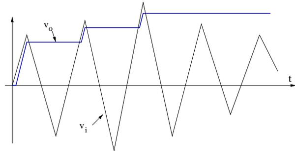
A practical peak-detector circuit includes a resistor in parallel with the capacitor. This resistor is either the load for the ideal peak detector or is placed in the circuit on purpose as is seen later.
