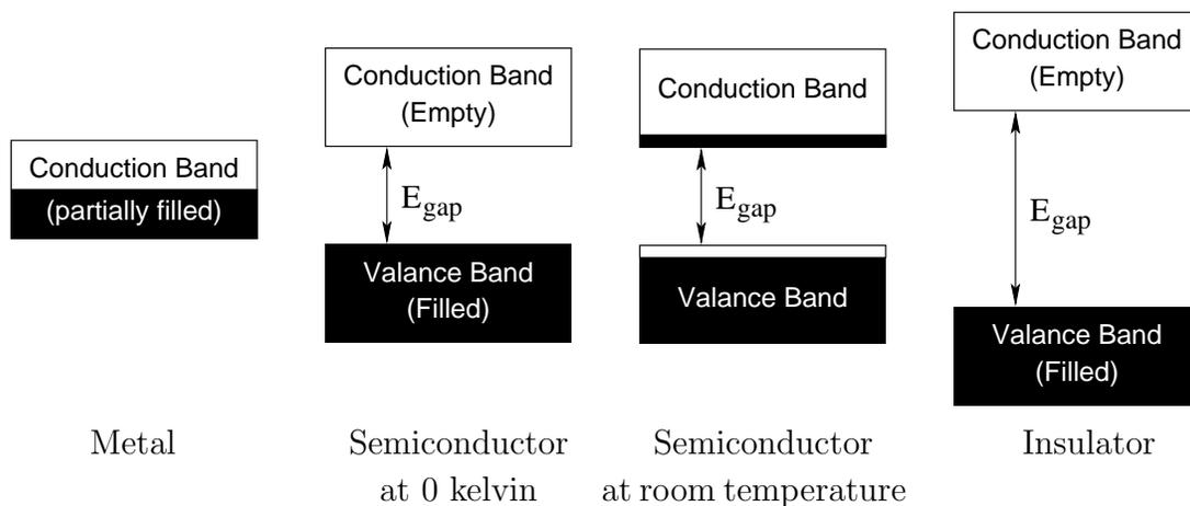
In metals, the conduction band is partially filled. As electrons in the partially filled conduction band can easily move around the material, metals can conduct electricity (and heat) very well.
