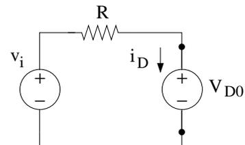
Therefore, the diode is ON with  $v_D = 0.7\text{ V}$  and  $i_D = 4.3\text{ mA}$ .
