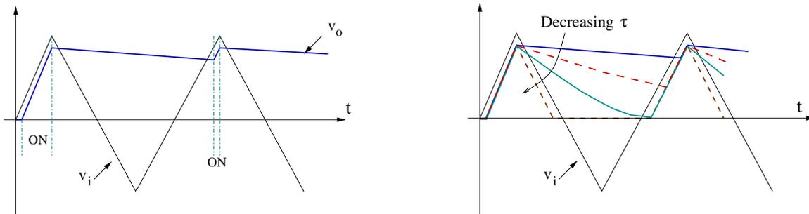
The shape of output waveform depends on how much the capacitor discharges in each cycle (see figure above right). For  $\tau = RC = \infty$ , capacitor does NOT discharge and we recover the ideal peak detector response ( $R = \infty$ ). Denoting the period of the input by  $T$ , if  $\tau \gg T$ , the capacitor would discharge very little in each cycle and  $v_o$  would be very close to that of an ideal peak detector.
