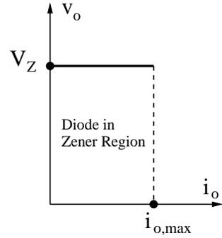
*Case 2: Diode is in the reverse bias region.* Let consider what happens if we exceed the  $i_{o,max}$ . The equivalent circuit is shown and we need to have  $-V_Z < v_D < V_{D0}$ . Because  $i_D = 0$ , KCL gives  $i = i_o$ . Then, KVL in the outer loop gives:
