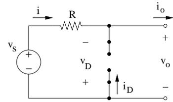
$$\text{KVL: } v_s = Ri_o + v_o \quad \rightarrow \quad v_o = v_s - Ri_o$$
