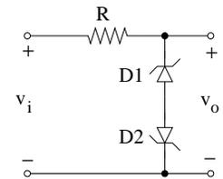
**Problem 16.** Consider a sinusoidal source with  $v_i = 15 \sin(\omega t)$  V. Design a clamp circuit that adds a DC offset of  $+5$  to the input voltage using a) DC power supplies only, b) Zener diodes only.
