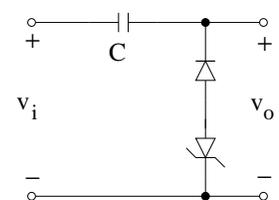
Capacitor values (or the load) should be chosen such that  $R_L C = \tau \gg T$ .
