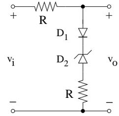
If D1 is ON,  $i_{D1} \geq 0$ . This means that  $i_{D2} < 0$  and D2 diode has to be in Zener state.
