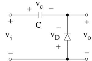
Similarly, we can produce different values of upward shift by the addition of a DC voltage source in series with the diode or using Zener diodes.
