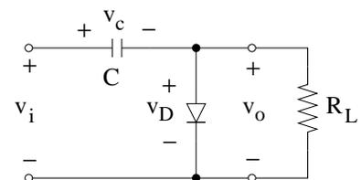
In a clamp circuit  $v_o = v_i - v_c$  and we need  $v_c$  to remain fairly constant in order for  $v_o$  to be a “shifted”  $v_i$  (and not distorted). Therefore, capacitor should discharge very little in each cycle. This constraint requires that  $\tau = R_L C \ll T$ . With this constraint,  $v_o$  of a clamp circuit with a  $R_L$  would be similar to that of the open-loop case.
