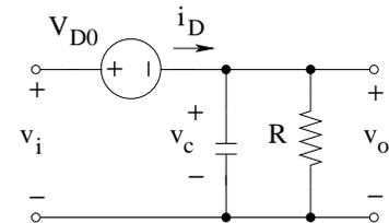
*Diode OFF:*  $i_D = 0$ ,  $v_D < V_{D0}$ : In this case we have an RC circuit with the capacitor discharging in the resistor with a time constant  $\tau = RC$  according to  $v_o(t) = v_c(t) = v_{c0} \exp[-(t - t_0)/\tau]$ .  $v_{c0}$  denotes the capacitor voltage when diode turned OFF (at  $t_0$ ). Diode remains OFF as long as  $v_D = v_i - v_c \leq V_{D0}$  or  $v_i \leq v_c + V_{D0}$ .
