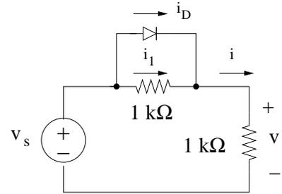
**Problem 10.** Find transfer function of the circuit below (Si diodes with  $V_{D0}=0.7$  V and  $V_Z = 5$  V for Zener diodes).
