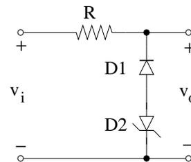
The above two circuits above can be combined to clip both voltages larger than  $v_{DC1} + V_{D0}$  and voltages smaller than  $-v_{DC2} - V_{D0}$ .
