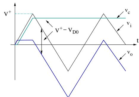
Let’s consider the impact of a load,  $R_L$ . During the first cycle when the diode is ON, the capacitor charges to a voltage of  $v_c = V^+ - V_{D0}$  (similar to open-loop case). However, when the diode turns OFF, the capacitor discharges in  $R_L$  and its voltage drops. Similar to a peak detector with a load, the diode turns ON in the following cycle and charge the capacitor back to  $v_c = V^+ - V_{D0}$ .
