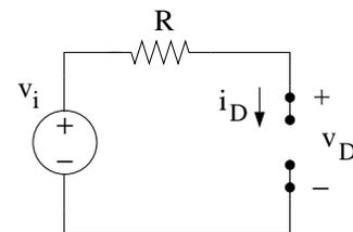
**Diode ON:** from the circuit by Ohm's Law,  $i_D = (v_i - V_{D0})/R = 4.3\text{ mA}$ . Since  $i_D > 0$ , our assumption is correct.
