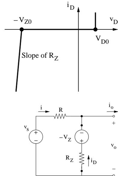
*Diode is in the Zener region:* The equivalent circuit is shown and we need to have  $i_D \leq 0$ . We assume that  $i_o$  is known and compute  $v_o$  (to get the response of the circuit) and  $i_D$  (to check for the diode state). KCL and KVL in the left loop give:
