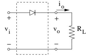
*Diode OFF:*  $i_D = 0$ ,  $v_D < V_{D0}$
