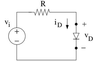
*Step 2:* Assume diode is OFF,  $i_D = 0$  and  $v_D < V_{D0}$ . Substituting for  $i_D = 0$  in the circuit equation, we get:
