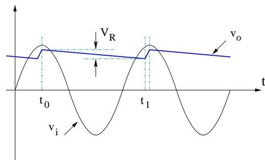
Obviously capacitor value should be chosen such that  $\tau = RC \gg T$ . For this application,  $R$  is the load (*i.e.* equal to  $v_o$  divided by the current drawn by the electronic circuit).
