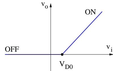
The figure below (left) shows how  $v_o$  can be found for a time dependent  $v_i$  (triangular wave in this case). We first find “time intervals” in which diode is OFF ( $v_i < V_{D0}$ ) and time intervals in which diode is ON ( $v_i \geq V_{D0}$ ): separated by vertical dashed lines in the figure. We can then construct the output wave-form by plotting  $v_o = 0$  when diode is OFF and  $v_o = v_i - V_{D0}$  when diode is ON as is shown below.
