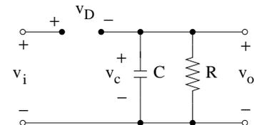
The diode OFF case is different from that of an ideal peak detector, as the voltage across the capacitor changes. The transfer function of the circuit is:
