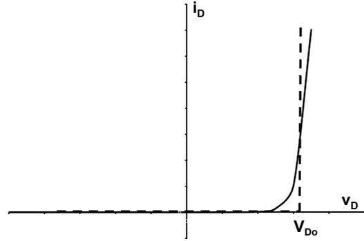
As can be seen from the figure, it is NOT possible to approximate the  $iv$  curve with ONE line. However, it is possible to do so with TWO (or more) lines. This type of approximation is called a piecewise linear model, *i.e.*, pieces of the curve are replaced by lines. One such model for diodes, called the “constant voltage model,” is shown in the figure with
