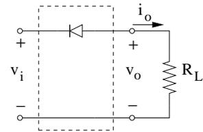
The above circuit is a simple method to convert AC input voltages to a “DC” output voltage and is used in AC to DC converter part of power supplies. Such circuits are called “rectifier” circuits. Because the output of the circuit above is only one half of the input waveform (figure below left), this circuit is called a “half-wave” rectifier circuit.
