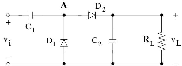
Capacitor C1 and diode D1 form a clamp circuit. As a result the voltage at point A is a sinusoidal voltage with a DC offset of  $V_p$  (ignoring  $V_{D0}$ ). Diode D2 and capacitor C2 form a peak-detector circuit. They will generate a DC signal with a value which is equal to the peak of AC signal or  $2V_p$
