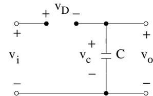
$$\begin{aligned} \frac{dv_i}{dt} \geq 0 \quad \& \quad v_i = v_c + V_{D0} \quad \text{Diode ON:} \quad v_o = v_c = v_i - V_{D0} \\ v_i < v_c + V_{D0} \quad \text{Diode OFF:} \quad v_o = v_{c0} \end{aligned}$$
