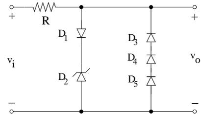
**Problem 14.** Design a clipper circuit that clips voltages above 5 V and below  $-3$  V using
