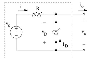
*Case 1: Diode is in the Zener region.* The equivalent circuit is shown and we need to have  $i_D \leq 0$ . KVL in the right loop gives:
