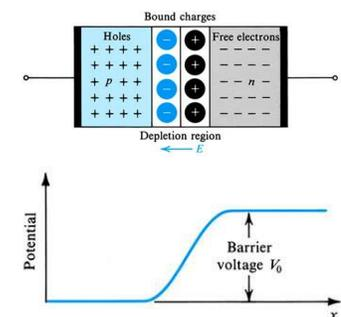
Since the n side has lost electrons, it becomes positively charged. Similarly the p side becomes negatively charged. As a result, an electric potential and an electric field appear across the depletion region. This voltage barrier impedes the flow of electrons from the n side and flow of holes from the p side, forcing  $I_{diff}$  to go to zero. The height of this voltage barrier is called the "junction built-in voltage."
