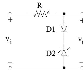
As power supplies are bulky and expensive, a Zener diode can be used instead of  $v_{DC}$  as is shown above (right). The draw back of a clipper circuit with Zener diodes is that  $V_Z$  is always positive. Therefore, we can only clip voltages above the positive value of  $V_{D0} + V_Z$ . The circuit containing the voltage source  $v_{DC}$  would allow clipping voltages above a “negative” value by choosing a negative  $v_{DC}$ .
