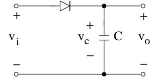
Using diode circuit models, we will arrive at circuits below. Note that  $v_o = v_c$ .
