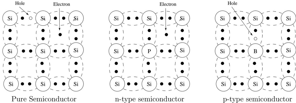
Similarly, we can create a p-type semiconductor by adding an element from group IIIB, such as B, to the semiconductor. In this case, the p-type dopants or the acceptor atoms, lead to a large number of holes. For p-type semiconductors, holes are majority carriers and electrons are minority carriers.
