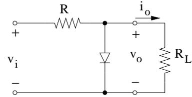
It is of interest to build circuits which can “clip” the input signal at values different than  $V_{D0}$ . These circuits can be realized by inspecting the clipper circuit above. We see that the signal is clipped when the diode is ON. At these time intervals, the diode appears as an independent voltage source in the circuit with  $v_o = v_D = V_{D0}$ . As such, Addition of a voltage source in series with the diode will change the clipping as is shown below. Note  $v_o = v_D + V_{DC}$ .
