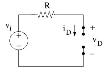
**Diode ON:** from the circuit by Ohm's Law,  $i_D = (v_i - V_{D0})/R$ .
