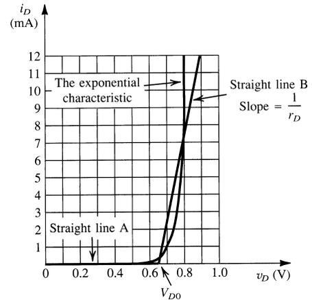
This type of model is useful only if resistances in the circuit are of the same order as  $R_D$  (typically  $10^3 \Omega$ ).
