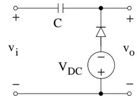
**Part B:** Prototype of circuit is shown with  $v_o = v_i + (V^- - V_{D0} - V_Z)$ .
