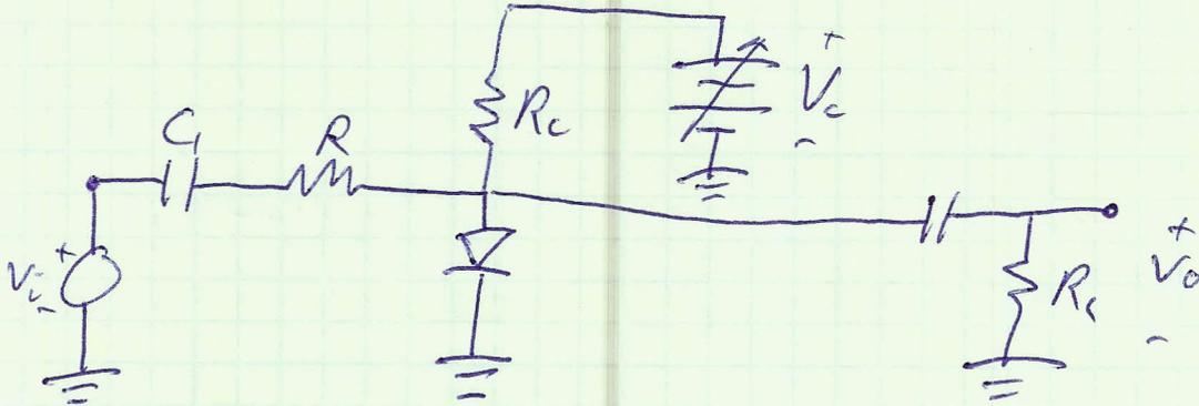
$$\text{Bias: } I_D = \frac{V_C - V_{D0}}{R_C}$$
