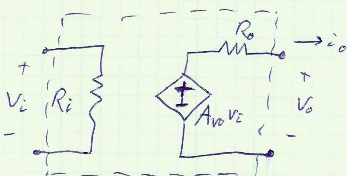
Can solve any amplifier circuit once to determine these parameters
