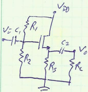
$$R_G = R_1 \parallel R_2$$
