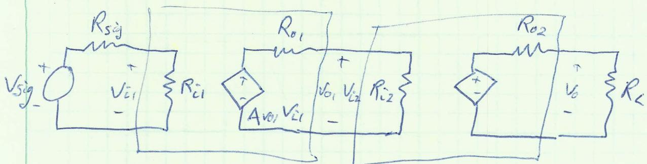
$$\frac{V_0}{V_{\text{sig}}} = \frac{R_{i1}}{R_{i1} + R_{\text{sig}}} \times A_{v1} \times \frac{R_{i2}}{R_{i2} + R_{01}} \times A_{v2} \times \frac{R_L}{R_L + R_C}$$
