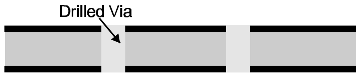
Figure 4.1.2 Holes drilled to define the locations of the vertical connections
