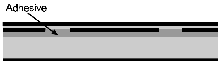
Figure 4.2.3 Two sheets bonded with an adhesive
