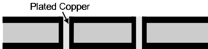
Figure 4.1.3 Plated copper forming vertical interconnections
