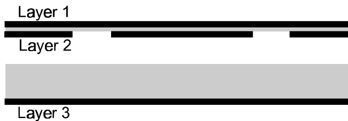
Figure 4.2.2 Inner layers patterned by etching
