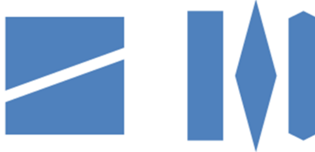
Figure 2.4: Unit cell examples. A square unit cell with a slit is shown on the left. Three different unit cells with two symmetry planes are shown on the right.
