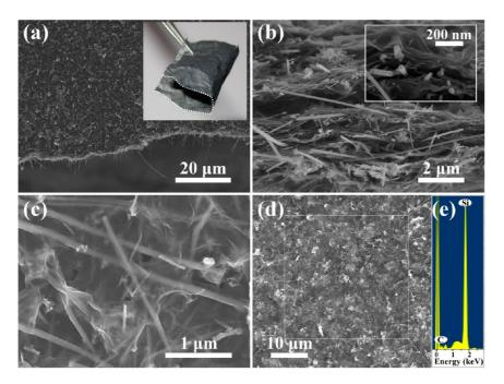
Figure 3. Characterization of SiNW@G@RGO: (a) low magnification SEM image. The inset shows an optical image of a bent SiNW@G@RGO film with a dashed line highlighting its edges. (b) Cross-section and (c) top-surface SEM images. The inset of panel b shows an enlarged cross-section view. (d) The corresponding region for collecting EDX spectrum in (e).
