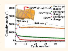
conductive RGO overcoats accommodate the volume change of embedded SiNW@G nanocables and thus maintain the structural and electrical integrity of the SiNW@G@RGO. As a result, the SiNW@G@RGO electrodes exhibit high reversible specific capacity of 1600 mAh  $g^{-1}$  at 2.1 A  $g^{-1}$ , 80% capacity retention after 100 cycles, and superior rate capability (500 mAh  $g^{-1}$  at 8.4 A  $g^{-1}$ ) on the basis of the total electrode weight.
