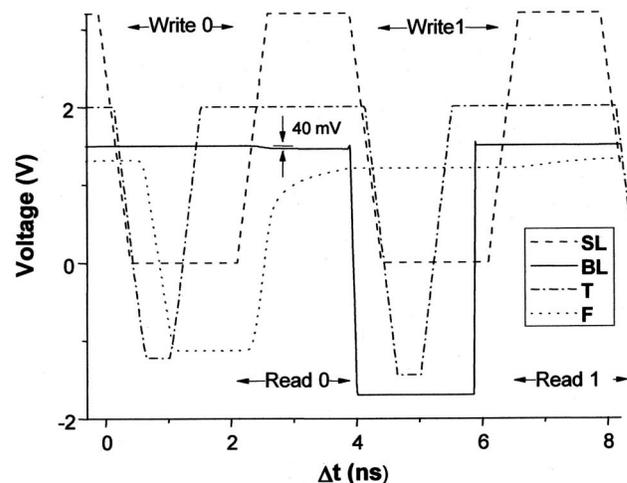
FIG. 2. Circuit simulations, at 0.25 GHz, for two read/write cycles of the proposed CNT based nonvolatile memory cell. The voltage of the sense line (SL), bit line (BL), write tip ( $T$ ) are systematically asserted to write and read logical values of 0 and 1 onto the floating conductor ( $F$ ).
