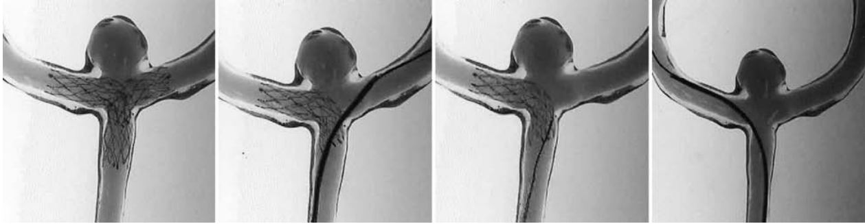
FIG. 2. Photographs depicting sequential placement of the stents in a Y-configuration across the aneurysm neck.
