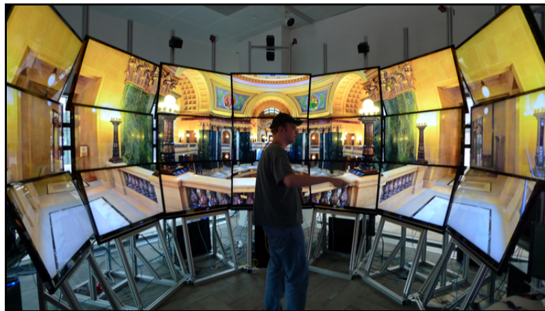
Figure 8. The NexCAVE high-resolution VR display at King Abdullah University of Science and Technology [10] presents polarized images matching the left and right views.
