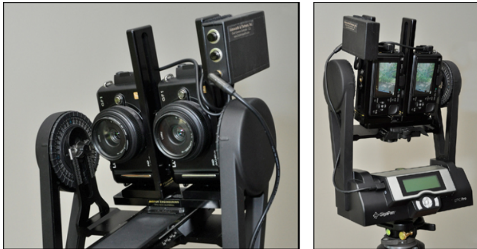
Figure 2. The dual-camera system is fully automated and can capture any number of stereo images covering a complete sphere or rectangle. Both nadir and zenith can be included, with the exception of a small footprint below the tripod.
