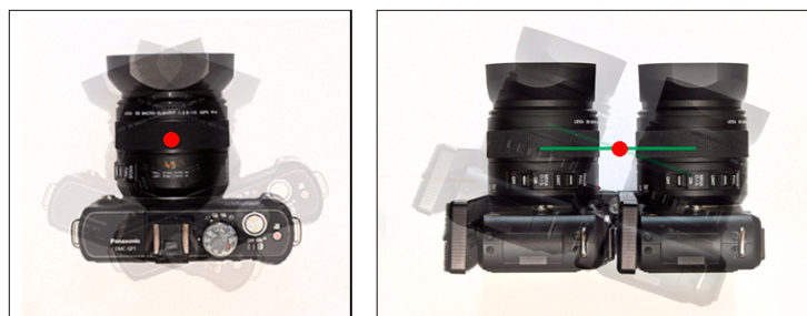
Figure 3. The left camera is rotated about the point of zero parallax to create a 2D image. The dual-camera stereo system on the right is rotated around a central point that is midway between the zero parallax points of the two lenses.
