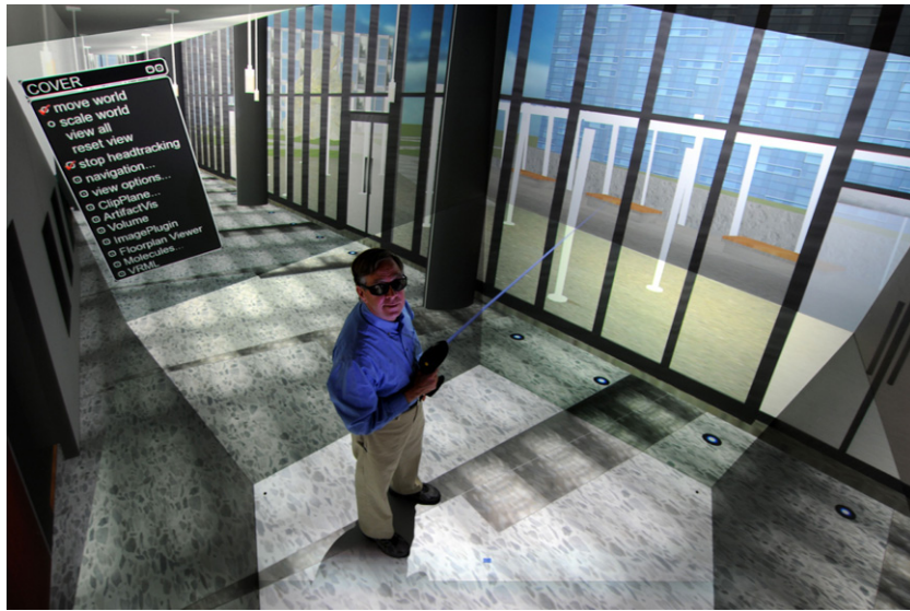
Fig. 3. A photograph taken with the camera being tracked of the simulated interior of the Calit2 Building at UCSD. Note the minimal seams, excellent perspective rendering, and the effect of the floor. Effects of vignetting and off-axis viewing are seen here as well, far more noticeable in still photographs than perceived when experienced live.
