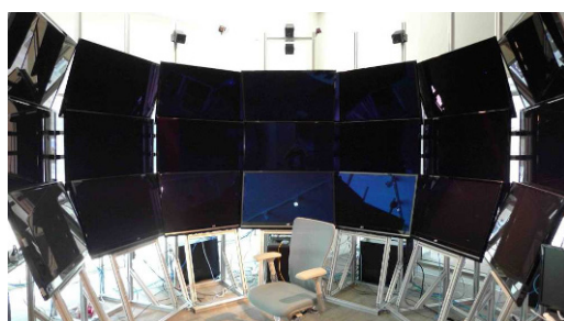
Figure 15. The KAUST NexCAVE turned off to show the structure designed and built by Greg Dawe. Photo: Tom DeFanti.
