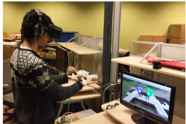
FIGURE 12: USER WEARING THE HAPTIC GLOVE AND OCULUS RIFT AND PLAYING THE PIANO IN VIRTUAL REALITY ENVIRONMENT WITH AUDIO AND HAPTIC FEEDBACK.
