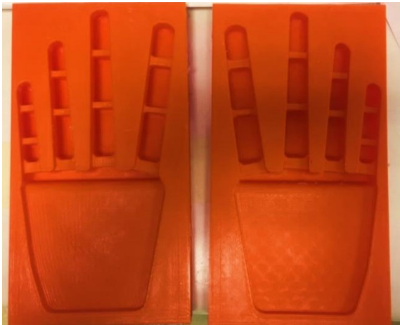
FIGURE 9: 3D PRINTED MOLDS FOR THE EXOSKELETON FOR LEFT AND RIGHT HAND
