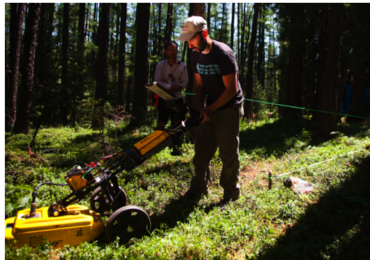
Fig. 1. GPR survey of this study’s field site in Northern Mongolia with the IDS dual frequency antenna detector.
