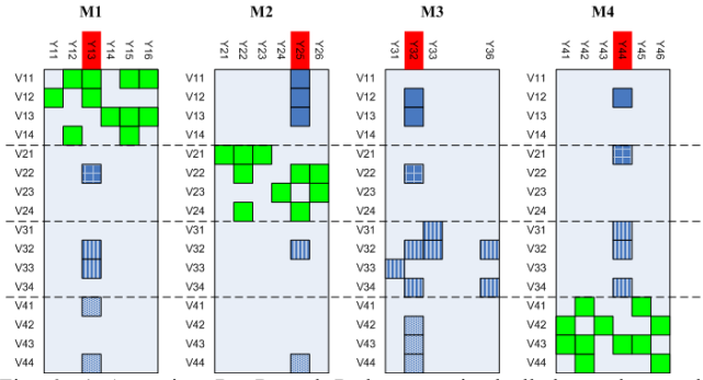
Fig. 6. a) Assuming R_1 , R_2 and R_4 have received all the packets and successfully recovered their original data (marked as green), but R_3 lost two code packets: Y_{34} and Y_{35} and need help.
