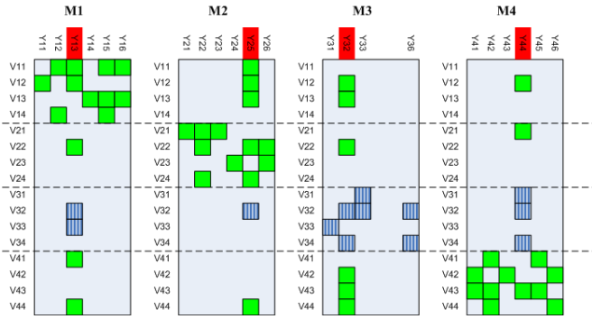
Fig. 6. b) The decoded original data packets are distributed to each other via pipe packets, and all pipe packets columns now become regular columns of M_3 .
