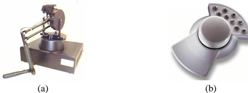
Figure 2.9: Mechanical tracking devices: (a) Phantom (b) Space Mouse.
