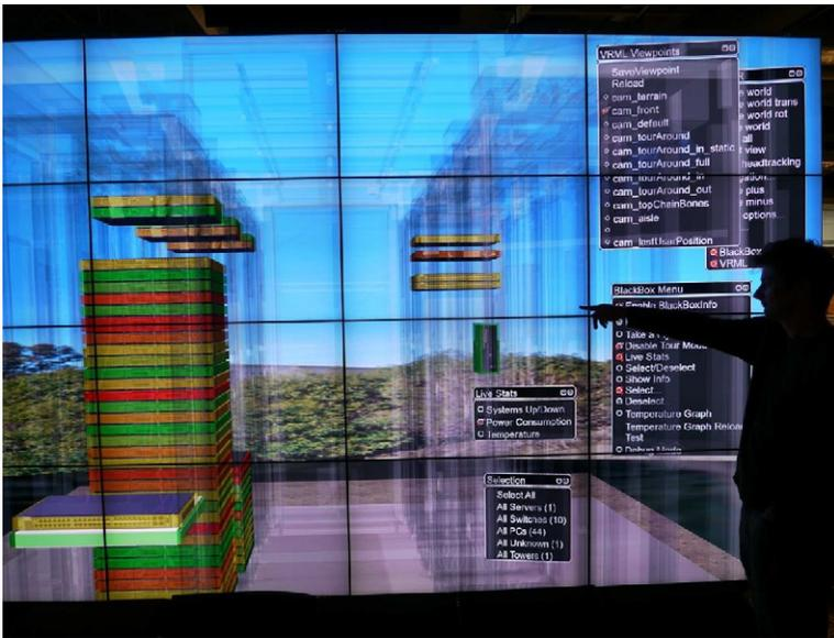
FIG. 3. AESOP Wall: 16 large, monoscopic narrow-bezel LCD displays with tracking and sound.
