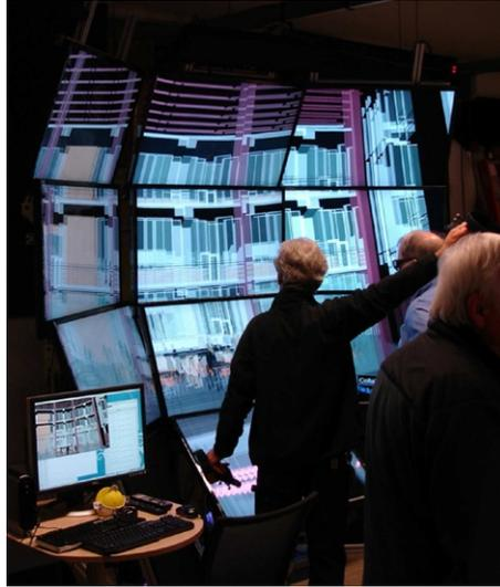
FIG. 2. NexCAVE: 10 overlapping passive stereo LCD displays.
