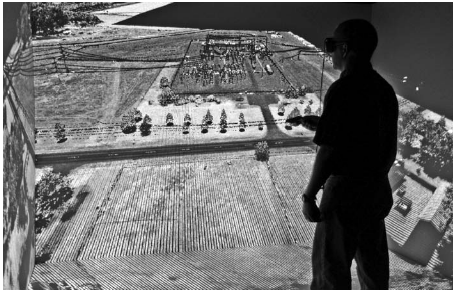
FIGURE 47.11 Data from an airborne LIDAR scan capturing the path of a powerline grid are presented using LidarViewer in a CAVE display.
