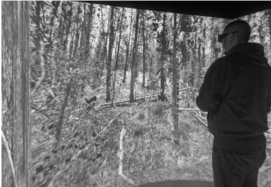
FIGURE 47.13 A user explores a wooded area captured by high-resolution LIDAR scans presented in a CAVE with LidarViewer.
