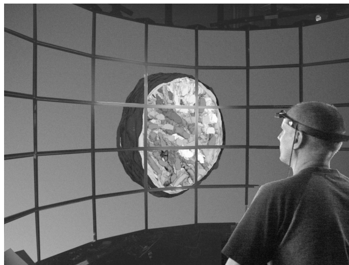
Figure 14.11 (a) illustrates how the barrier linescreen technology is used for generating pixel sets which are only visible to one eye at a time. Two such sets enable stereo vision. (b) shows a user interacting with the stereo display without using glasses.
