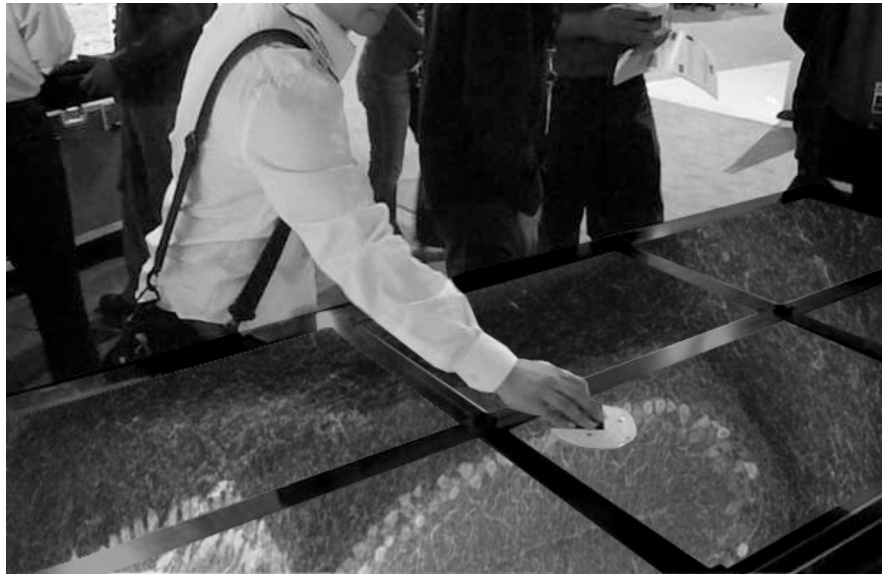
Figure 14.6 MagicCarpet running on the LambdaTable. The LambdaTable is a high-resolution, cluster-driven display table that supports multiple simultaneous users. (Image courtesy: Electronic Visualization Laboratory, University of Illinois at Chicago.)
