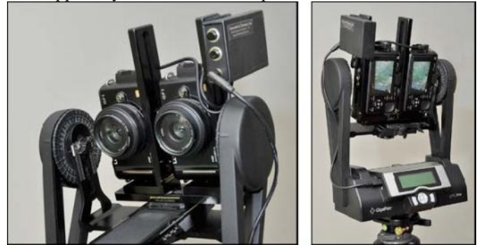
Fig. 1. The dual-camera system is fully automated and can capture any number of stereo images covering a complete sphere or rectangle. Both nadir and zenith can be included, with the exception of a small footprint below the tripod (Photo courtesy of Dick Ainsworth).
