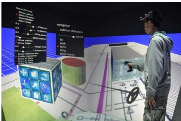
**Figure 3.** Using CAVE-CAD™ software architecture can be constructed around the viewer, immediately offering an experience of the design. Shown here are some of the tools (drop-down lists, palette cube) that have been implemented in the software.
