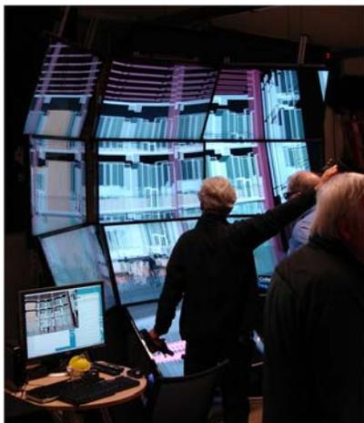
mounted to form an immersive VR system. The screens may be installed in a 3x3 array, which is curved towards the user in both directions, so as to maximize the coverage of the user's field of view. A 10<sup>th</sup> display is mounted below the center column to allow viewing the floor. The screens may be configured in larger arrays for enhanced peripheral views, larger content and CAVE like enclosure.
