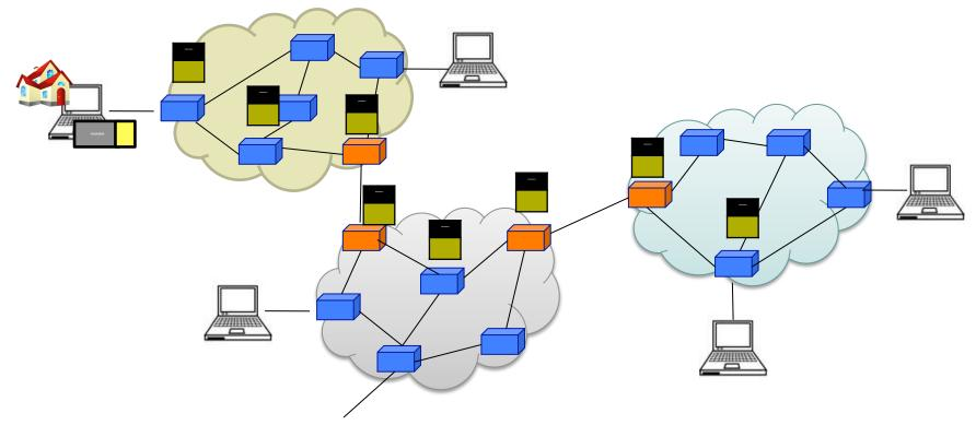
Hosts and routers are tied together by IP (Internet Protocol), a single common interface between users and the network and between networks
