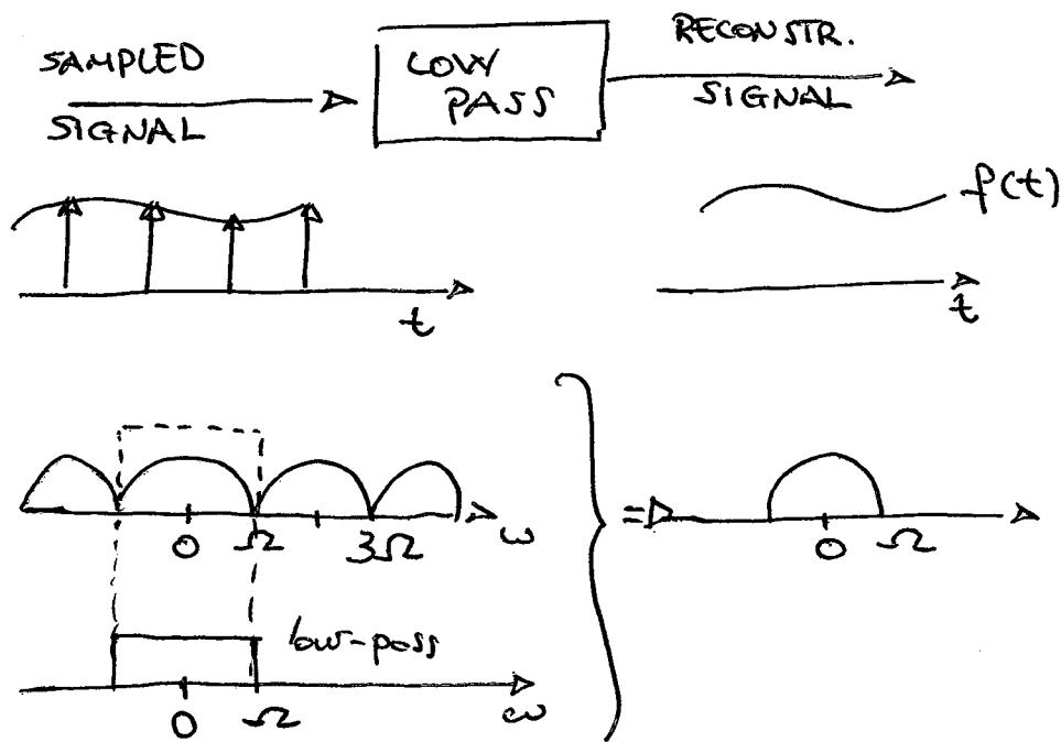
It follows that a signal of duration  $T_0$  can be reconstructed from  $\frac{T_0}{T}$  samples  $\frac{T_0}{T} = \frac{T_0 \omega}{\pi} = N_0$
