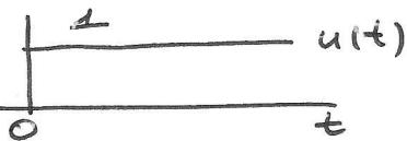
$$u(t) \xleftrightarrow{FT} \pi\delta(\omega) + \frac{1}{j\omega} \quad \begin{array}{l} \text{(This is shown at the end)} \\ \text{of lecture notes 9} \end{array}$$
