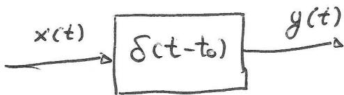
$$y(t) = \text{FT}^{-1} \left[ X(j\omega) e^{-j\omega t_0} \right] = x(t-t_0)$$
