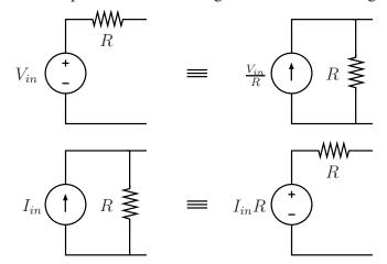
ullet Voltage/Current Divider: Application of KCL/KVL that allows for quick calculation of a voltage/current. For any  $n\geq 2$ .
