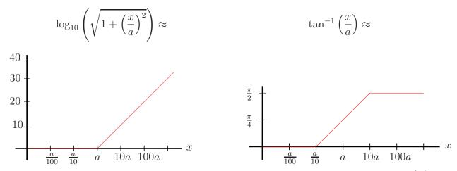
We can use these approximations to plot the magnitude and phase of a transfer function  $H(\omega)$ .
