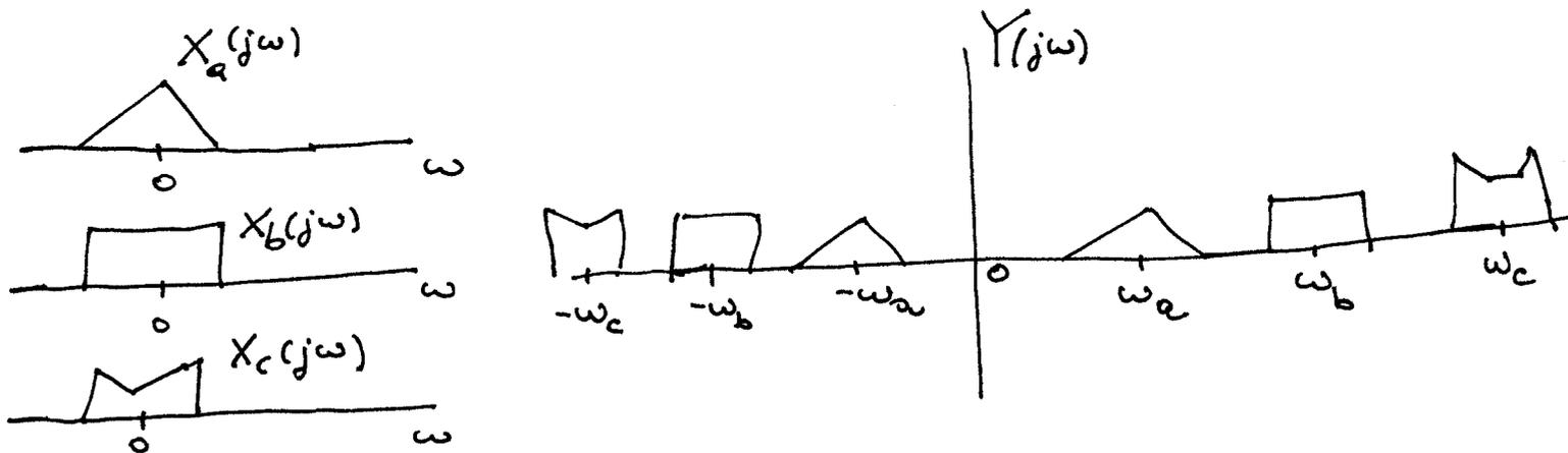
Suppose you have 3 radio stations each broadcasting their own signal, the signals are first modulated and placed in an appropriate frequency band and then broadcasted.
