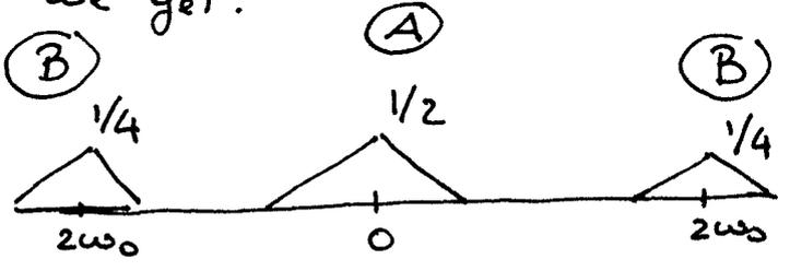
And after a low pass filter and multiplication by a factor 2 we obtain back the original signal.
