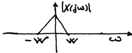
If samples of  $x(t)$  are taken sufficiently close together in relation to the highest frequency of the signal, then these discrete samples completely specify the entire signal
