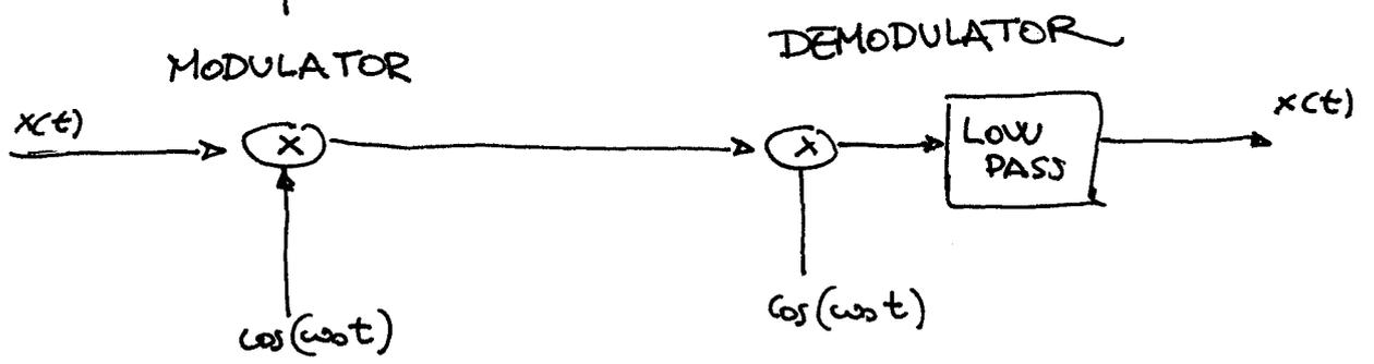
This is used to do Frequency Multiplexing of different signals:
