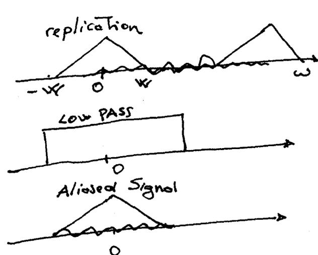
so when we low-pass this signal we still have some spurious high frequency components of the original signal that have been transferred in the low frequency regime and that we will hear as noise.
