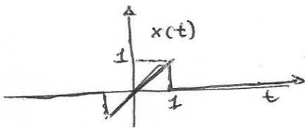
In general the derivative of discontinuity is a  $\delta$ -function of amplitude equal to the "jump" of the function
