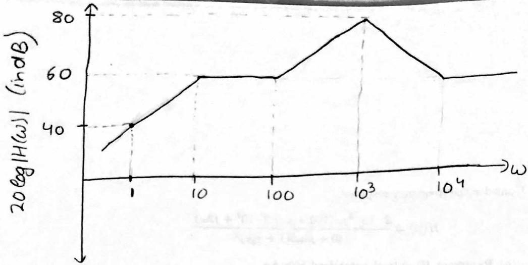
$$\angle H(\omega) = \frac{\pi}{2} + \tan^{-1}\left(\frac{\omega}{100}\right) + \tan^{-1}\left(\frac{\omega}{10^4}\right) - \tan^{-1}\left(\frac{\omega}{10}\right) - 2 \tan^{-1}\left(\frac{\omega}{10^3}\right)$$
