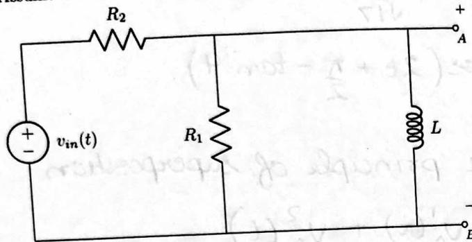
$$(R_1 = R_2 = 2\Omega, L = 2H)$$
