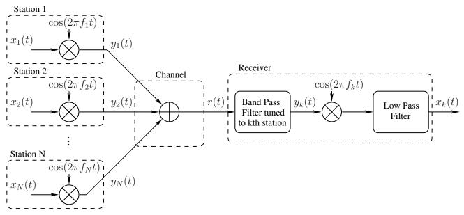
A block diagram of the basic amplitude modulation scheme used in this problem. Modulation allows for concurrent communication by dividing up portions of the frequency spectrum.
