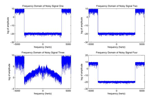
It can be seen that each signal has noise present in the frequencies in the range 3600 to  $F_s/2$ , but only signal 3 has a significant amount of frequency components in the range 0 to 3600. After applying a low-pass filter with cut-off frequency 3600 Hz, we obtain the following:
