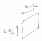
$$Ra = \gamma L^{3} \Delta T Par = 1.5 \times 10^{3} \times 0.5^{3} \times 20 \times 0.4 = 2.7 \times 10^{8}$$
