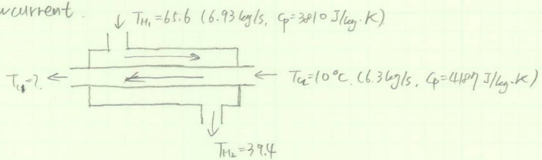
$$95\% \text{ ethanol: } \dot{Q} = \dot{m} c_p (T_{H1} - T_{H2}) = 691766 \text{ (W)}$$
