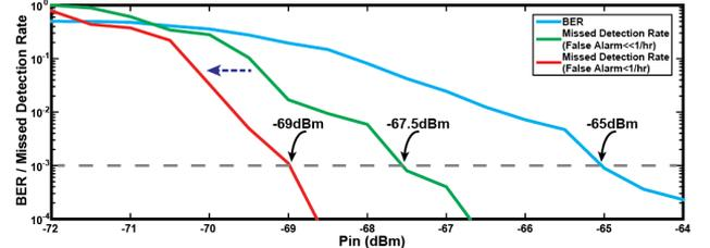
Figure 24.5.5: Measured power breakdown and waveforms with a correct pattern (top); BER & Missed-Detection-Rate curves (bottom).
