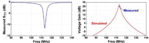
Figure 24.5.2: Schematic and 3-D model of the transformer; measured  $S_{11}$  and voltage gain.
