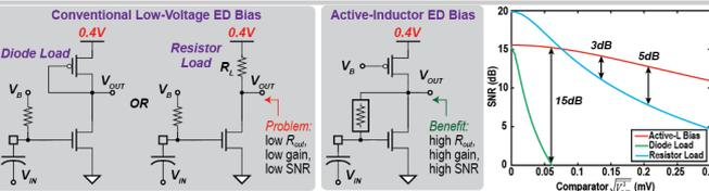
Proposed Low-Voltage DTMOS ED with Active-L Biasing:
