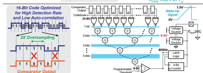
Figure 24.5.4: Dynamic comparator and S/H stage to eliminate kickback (top); 16b coding and digital correlator with output driver (bottom).
