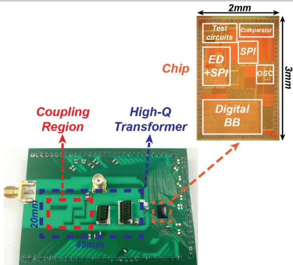
Figure 24.5.7: Die micrograph (top); photograph of the entire wake-up radio (bottom).
