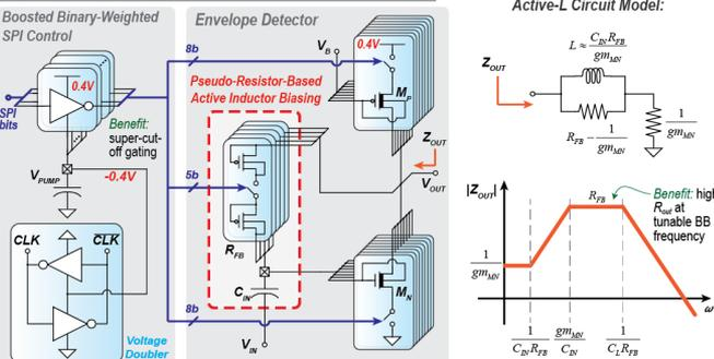
Figure 24.5.3: SNR comparison between three ED biasing schemes (top); active-inductor ED and equivalent output impedance (bottom).
