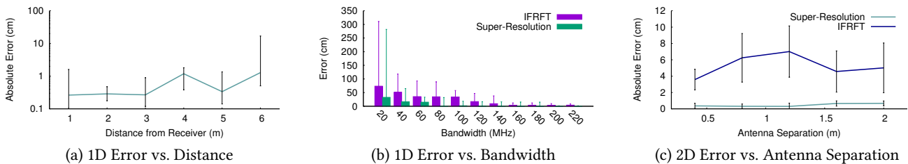
Figure 11: Micro-benchmarks. (a) shows that RFind’s accuracy gradually decreases with distance but the median error remains about 1 cm even at 6 m from the receiver. (b) shows that RFind’s accuracy increases with increased bandwidth both before and after super-resolution. (c) shows the independence of RFind’s accuracy from antenna separation. In each figure, error bars indicate 10^{th} and 90^{th} percentile accuracy.
